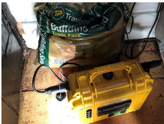
Figure 3.8: Vibration Monitor at 27 High Street (Inside)
